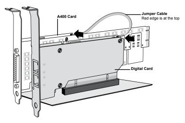
The digital card must have a hardware echo canceller installed. The minimum firmware that supports clock synchronization for the A400 is v10. For more information, please go to <a href="wiki.sangoma.com/t1e1analogfaxing">wiki.sangoma.com/t1e1analogfaxing</a>
